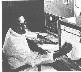
. . . mixed with chemicals which absorb any residues, and analyzed in a gas chromatograph.
