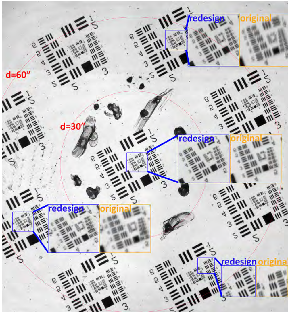
Fig. 5. Image of a test target obtained after the redesign. The blue insets show magnified sections, and the orange insets demonstrate the comparison to the original optics setup, which suffered from astigmatism and coma outside of the image center. The redesigned optics are perfectly sharp across the whole field of view. The image scale is indicated with red circles, whose diameters are specified in the figure.
